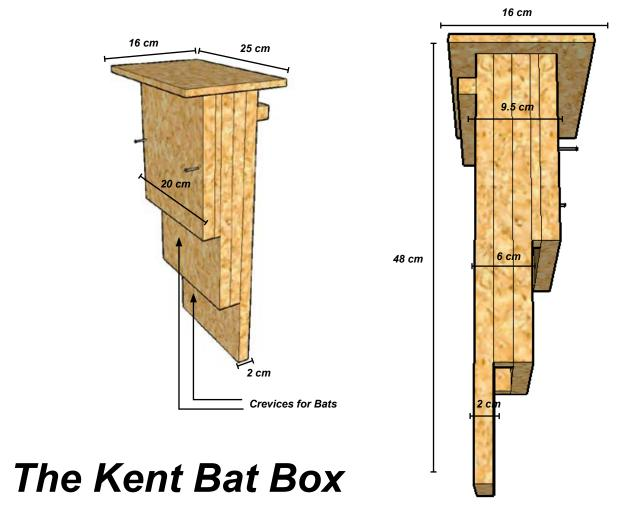
The box should be constructed from untreated rough-sawn timbers, with 2 or 3 crevices - the limiting factor being the weight and thickness of the box. The crevices may be any size between 15 and 25mm. Timber should be around 20mm thick. The box should be made to be rainproof and draught-free.
